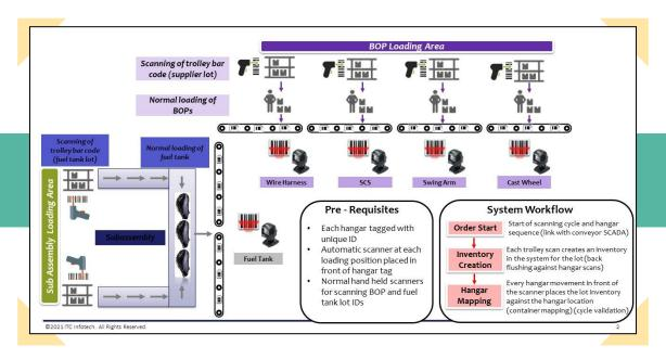
components are loaded on the line either in trolley or individually for critical components. Each trolley/component were scanned at line to provide the traceability. This implementation was done for main line and subassembly line as well.
